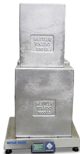
BC scale being tested at 500% of its capacity.
